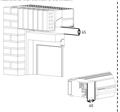
Apply the swellable tape (preferably: 15/2-6 swellable tape) to both sides and the bottom. Swellable tape is not to be applied to the top yet. Swellable tape needs to be applied to the inside and outside of the ventilator.
