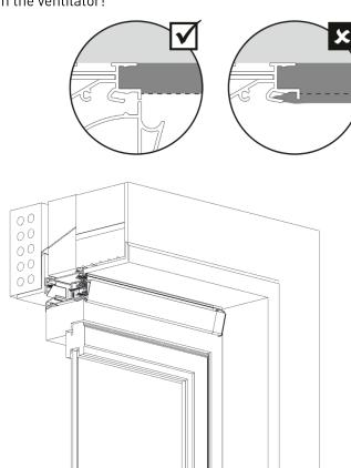
Seal off all joints and openings on the outside with a silicone sealant of choice.
