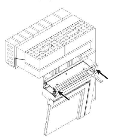
Fix the anchors to the structure (type of fixing dependent on the structure). If necessary, bend the end of the tie to do this. Check again to ensure that the ventilator is not showing any twist. Finish off the inside next to achieve a completely airtight seal.
